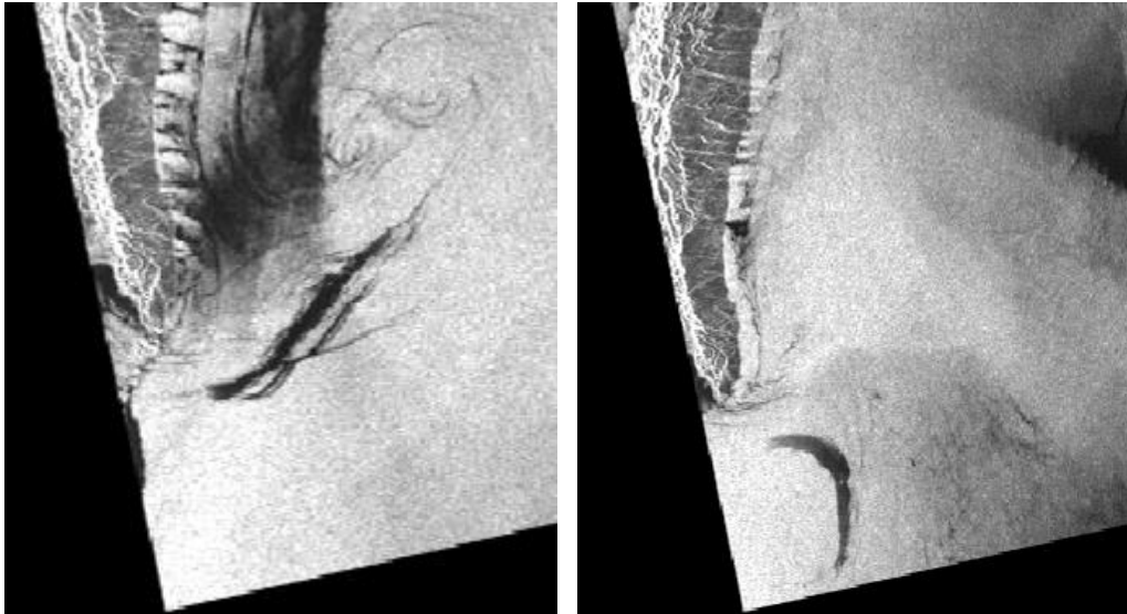
Figure 3 Repeating oil slick (dark linear feature) identified from Radar imagery over Lake Tanganyika. The two Radar images have been acquired on separate dates. The surface slick appears to share a common source point and is repeated on an additional 3 scenes over a 10 year period
