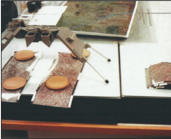
Stereoscope with prints of Landsat and declassified Corona imagery on light table
