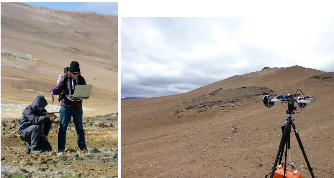
Figure 3: a) using an ASD Fieldspec Pro to collect in-situ VNIR spectra from targets within each region imaged by AUPE; b) AUPE in action
