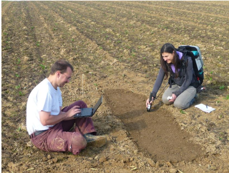
Figure 2: set up of erosion plots in the field (loess area, Limburg, Netherlands).
