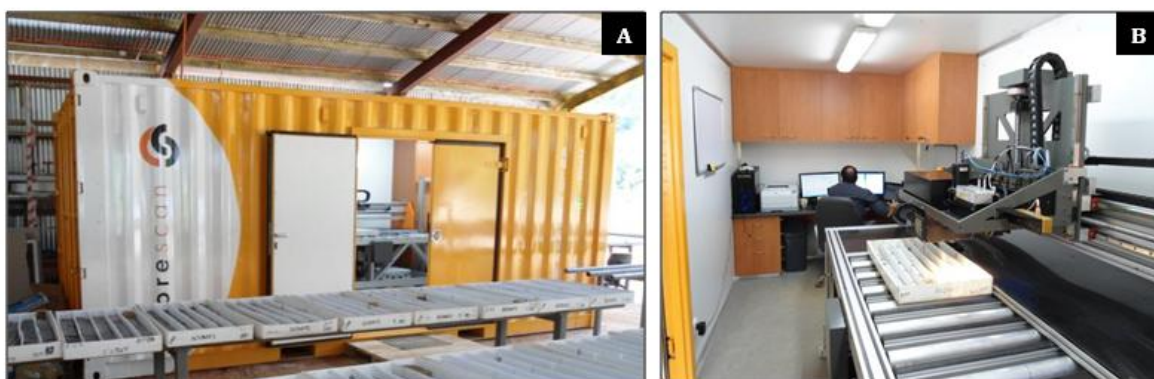
Figure 1: A. Mobile Corescan field lab; fully containerized in a standard 22' sea-tainer capable of transport by ship, air and road to any desired location including mine sites, drill pads, coresheds, etc. B. The Corescan system; core or cuttings are placed on the translation table while the three imaging systems (hyperspectral, RGB photography and laser profiler) scan over each length of core within the tray separately. A trained operator monitors the scanning, performing QC for all data in real-time.
